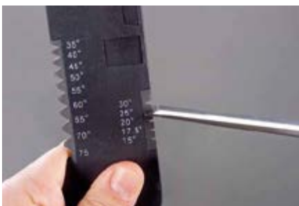
1. 检查并判定裁切角 Step 1: Check and determine the cutting angle.
