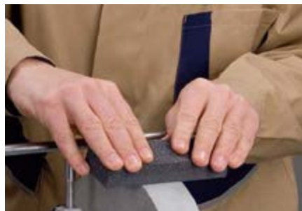
(粗/细) 修整砂轮 (Rough/fine) dressing of the grinding stone
