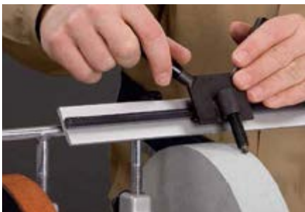
修整砂轮 Dressing the grinding stone
