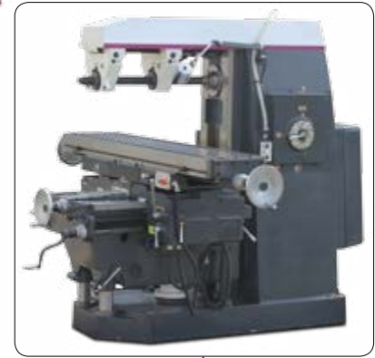
卧铣 Horizontal milling position
