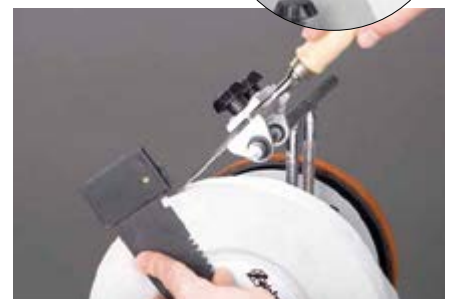
3. 设置裁切角度的匹配高度 Step 3: Set the matching height for the cutting angle.
