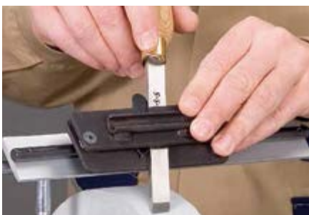
0-30°角度的研磨 Grinding at angles between 0-30°
