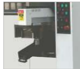
End remnant device (Optional, it can short the end remnant)
